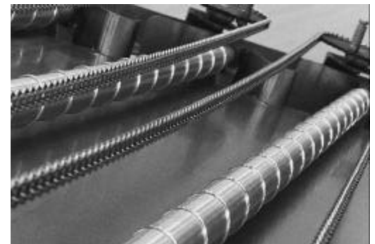
Revolving spiral rollers are raised or lowered to allow grading of different sizes.
