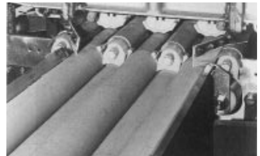
Shells are pulled through rollers away from edible meats.
