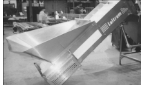
Loading shrimp into the Feed Conveyor Hopper is the only manual operation required until the Model IB Inspection Belt.
