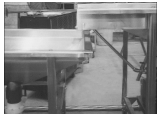
Cleaned shrimp are discharged from the Rock Tank into the Receiving Tank where the food pump gently sends shrimp to the Peeler.
