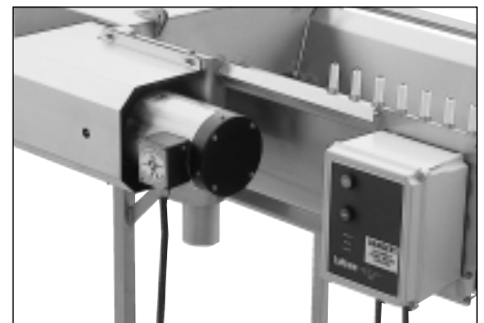
Drive motors are mounted away from processing area to insure minimal product contamination.
