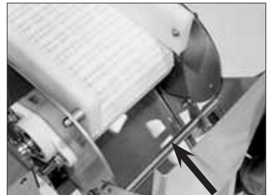
Water spray line at top of conveyor insures the complete discharge of shrimp.
