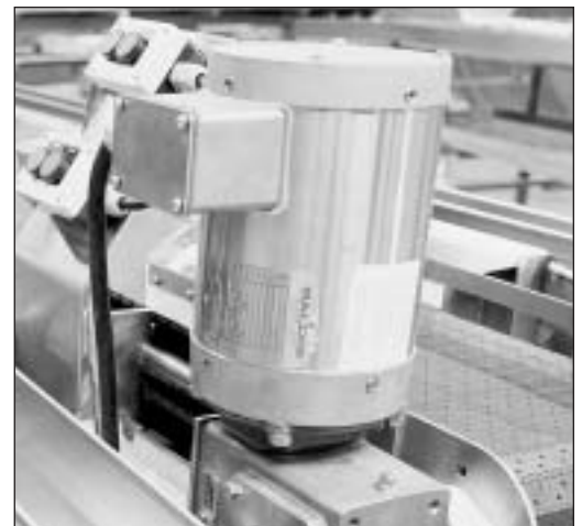
Variable speed motor allows operator to adjust conveyor belt speed.
