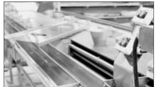
Removable table top and discharge chutes facilitate easy access for cleaning and sanitation.
