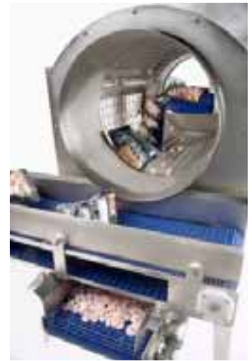
Contents of packaging pass through the drum's sieve for further processing.
