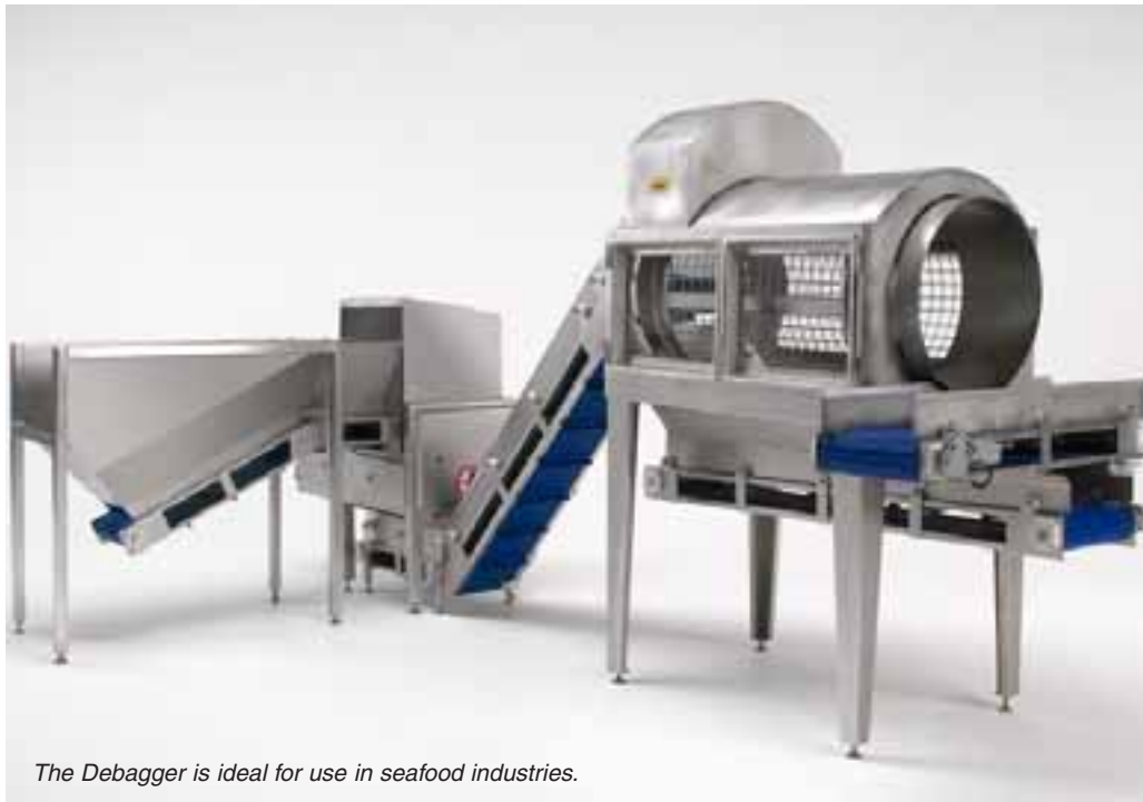
Contents of packaging pass through the drum's sieve for further processing.
