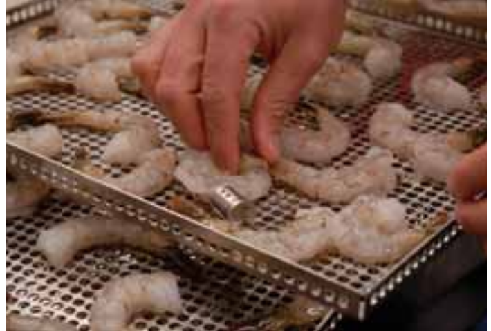
Mesa Labs' real-time data logger, the Micropack IV, being used during the shrimp cooking trials.
